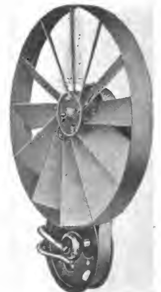
Fig. 15.—Example of the indiscriminate use of very many fan blades, a poor design.
